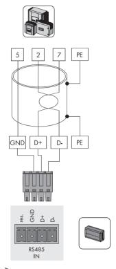
Insert the plug into the "RS485 IN" socket of the RS485 Power Injector.
