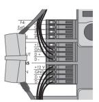
Connect the wires to the "F2: OUT RS485" terminals of the Sunny SensorBox. Note the configurations in your RS485 communication bus.
