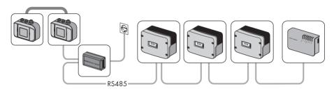
You can add an additional Sunny SensorBox to the Sunny SensorBox. If you do add another one, note that you can use the RS485 Power Injector to supply power to up to five Sunny SensorBoxes in total.
