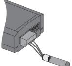
☐ The RS485 Power Injector is connected to the RS485 communication bus. You can now connect the RS485 Power Injector to the Sunny SensorBox.
