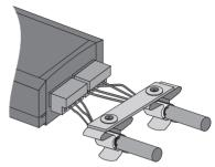
9. Route the RS485 communication cable from the RS485 Power Injector to the Sunny SensorBox.
