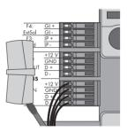
23. Connect the RS485 communication cable to the "F1: IN RS485" terminals of the Sunny SensorBox. Observe the noted wire colors.
