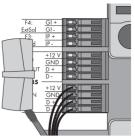
18. Connect the wires to the "RS485 F1: IN" terminal of the Sunny SensorBox. Observe the noted wire colors.
