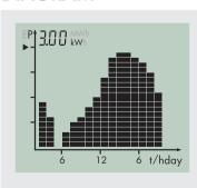
The inverter energy is shown as a diagram on the display. The daily graph is displayed by default. The right-hand flashing bar of the diagram represents the current hour. If the inverter does not feed any power to the grid over a longer period of time (e.g. in darkness or if the PV modules are covered with snow), a gap is inserted into the chart. The bar for the current hour is updated automatically every five seconds.
