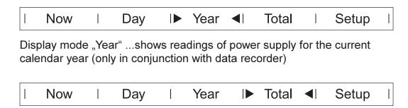
Display mode "Total" ...shows readings of power supply since original start of operation of the FRONIUS IG unit.
