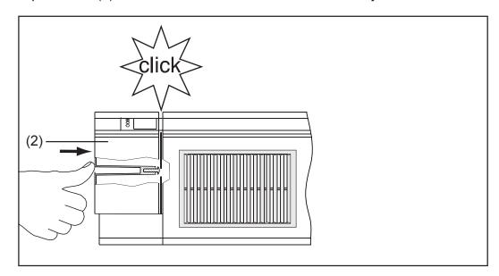
**Important!** To close the connection area put on cover (2) and push it forward until it reaches the locking position.
