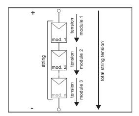
Power output and voltage are increased by combining a number of solar cells. If solar modules are connected in series like on a string, both the output potential as well as the voltage will increase.
