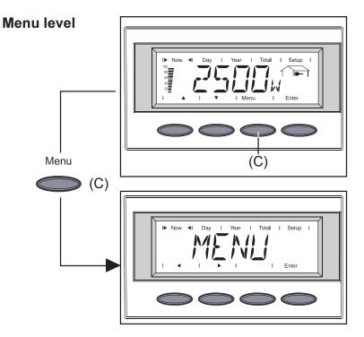
From the menu level you enter the display mode or the setup menu. Move into the menu surface by pressing key (C)
