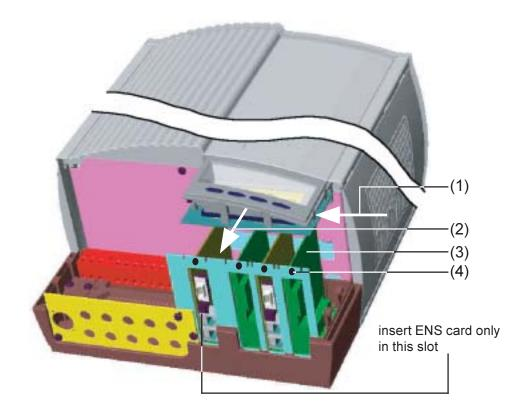
Insert slot-in boards, FRO-NIUS IG (Installation for indoor housing) (continued)
