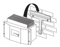
4. Secure the Sunny Boy in position fastening the supplied M6x12 screw.
