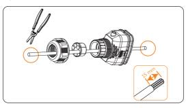
Figure 8-32 Stripping the communication cable for CT
