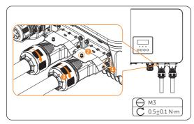
Figure 8-16 Installing the AC connector to inverter
