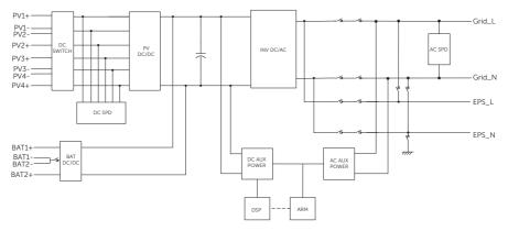
Figure 2-5 Circuit diagram for X1-VAST series inverter
