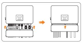
Figure 8-65 Pushing in the cable protective cover
