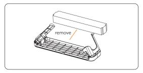
Figure 8-62 Removing the buffer material
