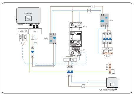
Figure 15-14 Connection diagram of Meter on EPS terminal
