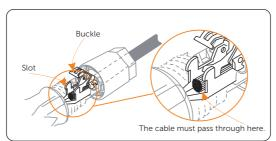
Figure 8-27 Diagram of buckle and slot
