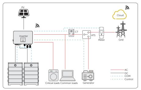
Figure 15-2 Dry contact wiring diagram
