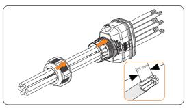
Figure 8-41 Threading the cables and stripping the insulation
