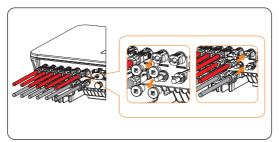
Figure 8-30 Connecting the battery connector
