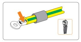
Figure 8-5 Crimping the cable
