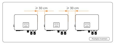
Figure 5-5 Clearance requirement for multiple inverters
