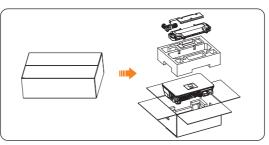
Figure 6-1 Unpacking the inverter (Australian version with cable protective cover)
