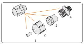
Figure 8-59 Disassembling the waterproof connector
