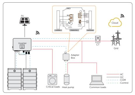
Figure 15-4 Adapter Box G2 wiring diagram
