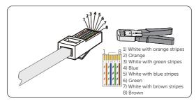
Figure 8-52 Crimping the communication cable
