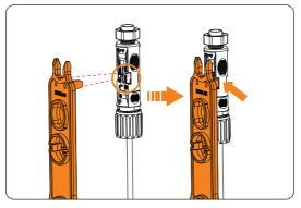
Figure 13-5 Disassembling the PV connector
