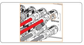
Figure 13-7 Disassembling the Battery connector
