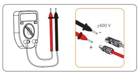
Figure 8-22 Measuring the voltage of PV connectors
