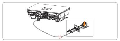
Figure 15-9 Connecting to EV-Charger
