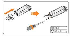
Figure 8-57 Assembling the dongle
