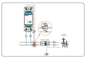
Figure 15-10 Connecting DDSU666-CT to the grid
