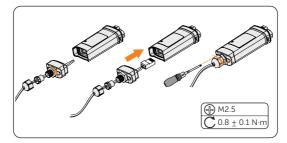
Figure 8-60 Assembling the dongle
