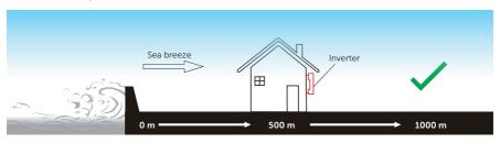
Figure 5-1 Recommended installation position
