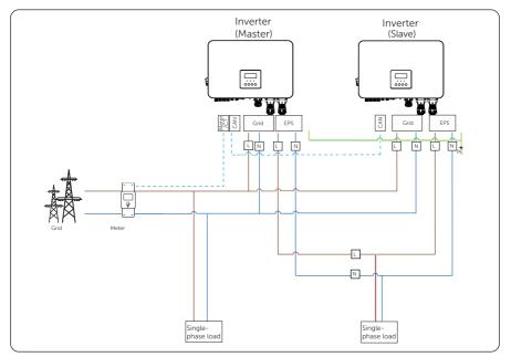
Figure 15-15 System wiring diagram
