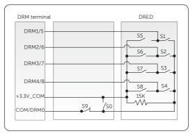
Figure 8-46 DRED connection diagram
