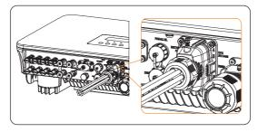
Figure 8-45 Connector connected
