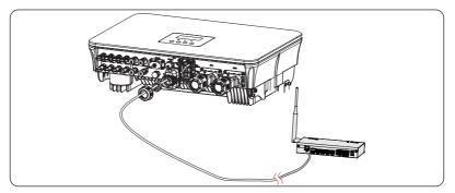
Figure 15-12 Connecting to DataHub
