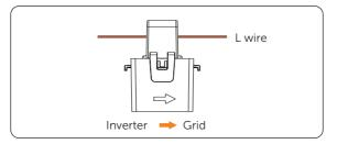
Figure 15-2 Clipping CT to grid cables
