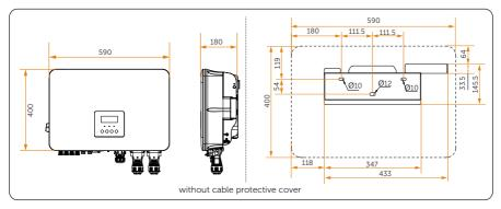
Figure 7-3 Dimensions (European version) (Unit: mm)
