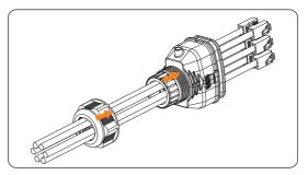
Figure 8-40 Threading the cables with RJ45 terminals
