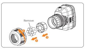
Figure 8-39 Disassembling the connector
