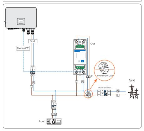
Figure 15-9 System wiring with SolaX DDSU666-CT
