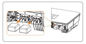
**Step 2:** Remove the dustproof cover of the Grid&EPS terminal.
