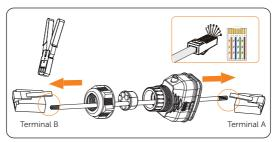
Figure 8-33 Crimping the communication cable for CT
