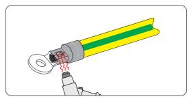
Figure 8-6 Shrinking the tubing
