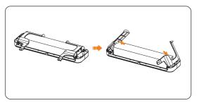
Figure 8-61 Opening the support frame
