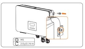
Figure 7-11 Securing the inverter with the wall-mounting bracket
