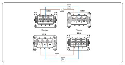
Figure 15-16 Power cable wiring
