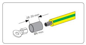
Figure 8-4 Installing the tubing and R-type teriminal
