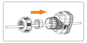
Figure 8-31 Threading the communication cable
