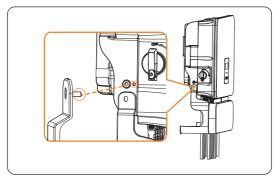
Figure 8-67 Left side cable protective cover installation
