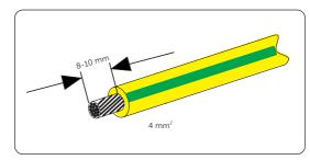
**Step 1:** Strip the insulation of the PE cable to an appropriate length.
