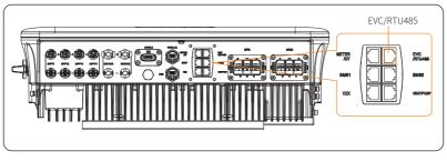
Figure 15-8 Connection terminal for EV-Charger
