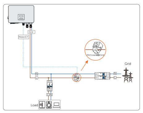
Figure 15-1 System wiring with CT
