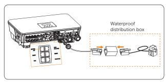
Figure 15-3 Connecting the inverter to the CT
