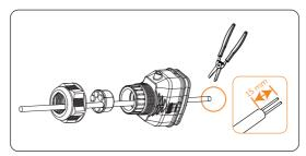
Figure 8-34 Stripping the communication cable for meter
