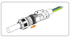
Figure 8-12 Threading the grid cable
