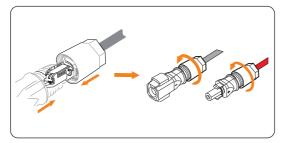
Figure 8-29 Tightening the swivel nut
