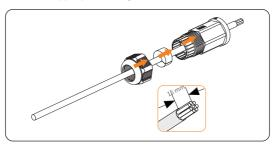
Figure 8-51 Threading the cables and stripping the insulation
