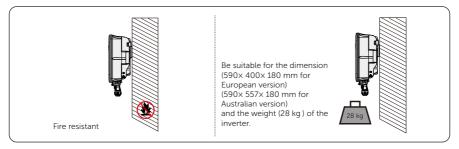
Figure 5-3 Installation carrier requirement
