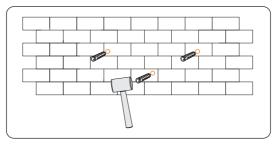
Figure 7-8 Knocking the expansion tubes Fixing the wall-mounting bracket
