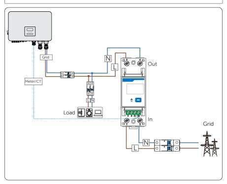
Figure 15-3 System wiring with SolaX DDSU666
