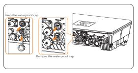
Figure 8-48 Loosening the waterproof cap
