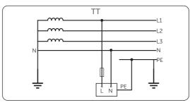
Figure 2-2 Supported power grid-TT
