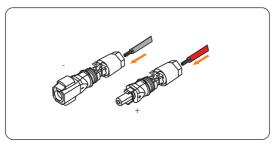
Figure 8-26 Inserting the battery pin contact
