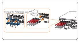
Figure 8-23 Connecting the PV cable
