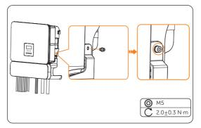
Figure 8-69 Right side cable protective cover installation
