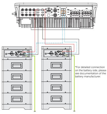
Figure 8-37 BMS connection diagram
