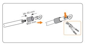
Figure 8-13 Crimping the conductors
