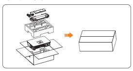
Figure 13-11 Packing the inverter (Australian version with cable protective cover)
