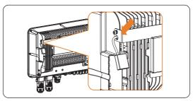
Figure 7-12 Locking the inverter
