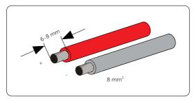
**Step 1:** Strip the insulation of the battery power cable to an appropriate length.
