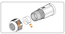
Figure 8-49 Disassembling the connector
