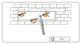
Figure 7-9 Fixing the wall-mounting bracket
