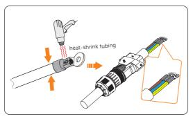
Figure 8-14 Shrinking the tubing
