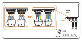
Figure 8-15 Connecting the AC cable
