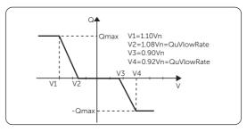
Figure 10-5 Curve Q = f(V)
