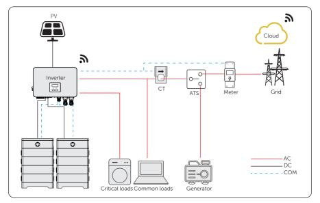
Figure 15-1 ATS control wiring diagram
