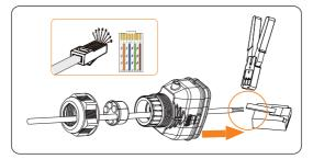
Figure 8-35 Crimping the communication cable for meter
