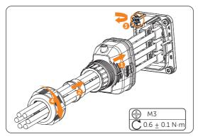
Figure 8-44 Securing the connector
