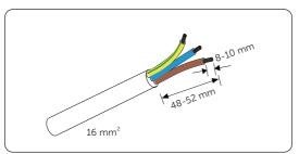
Figure 8-9 Stripping the Grid cable
