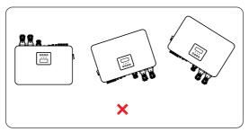
Figure 7-2 Incorrect installation
