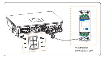
Figure 15-12 Connecting inverter to meter
