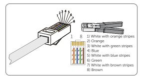
Figure 8-42 Crimping the communication cable
