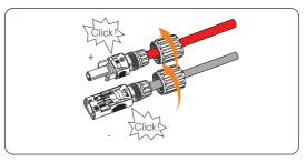
Figure 8-21 Securing the PV cable
