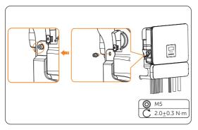
Figure 8-68 Left side cable protective cover installation
