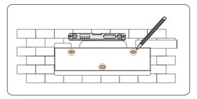
Figure 7-6 Marking the holes
