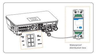
Step 3: Connect the conductors to terminal 24 and 25 of the meter.
