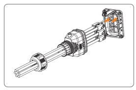
Figure 8-43 Installing the network cable to the cable terminal
