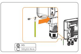
Figure 8-8 Securing the PE cable
