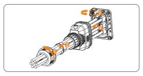
Figure 13-9 Removing COM connector
