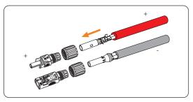
Figure 8-20 Threading the PV cable
