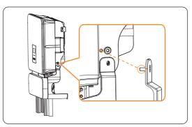
Figure 8-66 Right side cable protective cover installation
