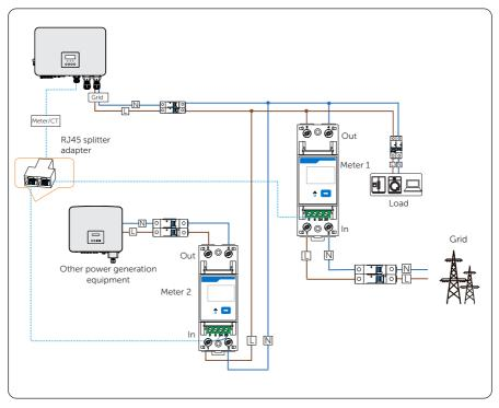
Figure 15-15 Connecting to double direct-connected meters
