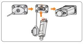
Figure 8-58 Dongle connection procedure
