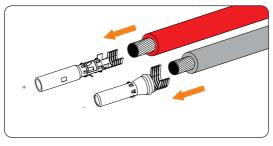
Figure 8-18 Inserting the PV pin contact
