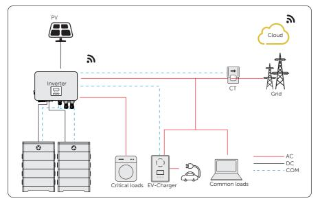
Figure 15-7 EV-Charger wiring diagram
