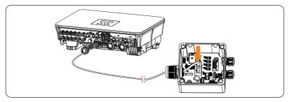
Figure 15-6 Connecting to Adapter Box G2
