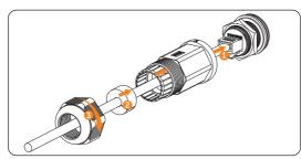
Figure 8-53 Securing the connector
