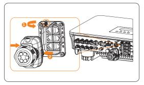
Figure 8-38 Removing the connector enclosure
