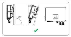
Figure 7-1 Correct installation
