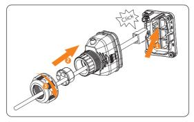
Figure 8-36 Connecting cable to the Meter/CT port
