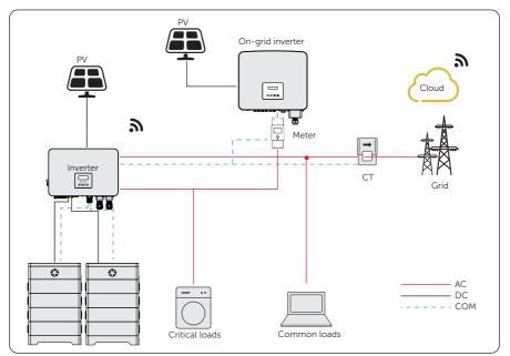
Figure 15-13 Micro-grid wiring connection
