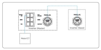
Figure 15-17 Communication wiring
