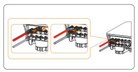
Figure 13-6 Disassembling the dustproof buckles
