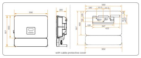
Figure 7-4 Dimensions (Australian version) (Unit: mm)
