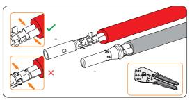
Figure 8-19 Crimping the terminal
