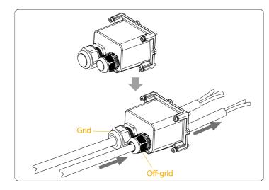
Step 3. Remove the 12mm insulation layer at the end of the wire. Insert the European-style terminals respectively, and make sure that the stripped ends are inserted into the European-style terminal ,and finally use crimping pliers to press tightly.
