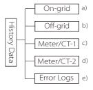
The history data contains five pieces of information: on-grid power of the inverter, off-grid power generation, power of the meter/CT and error Error logs.
