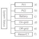
System status contains six content:PV1/PV2/Battery/On-grid (energy feed into or buy from the grid)and Off-grid and so on. Press up and down to select, press "Enter" to confirm the selection, and press "ESC" to return to the menu.
