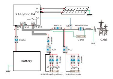
Diagram B: Neutral line and PE line are separated from each other, all loads connect to the Off-grid port; (For most countries)
