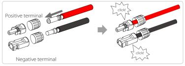
Step 6. Tighten the fastening head and into insert the corresponding positive and negative (PV-/PV+) ports of the inverter.
