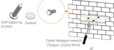
> Step 3: Tighten the inverter and bracket.
