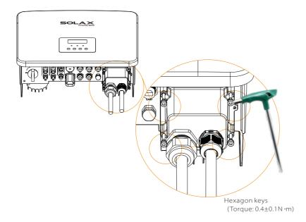
Step 6. Tighten the waterproof fastening head.
