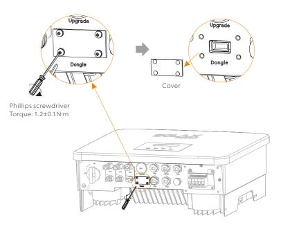
Step 2. Plug the Pocket WiFi Plus into the DONGLE port, use the screws in the Pocket WiFi Plus accessory to tighten it.
