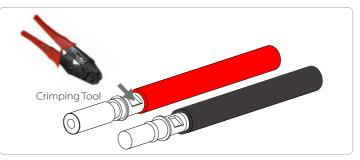
Step 5. The PV joint is divided into 2 parts - the plug and the fastening head. Insert the cable through the fastening head and the opposite plug. Note that the red and black lines correspond to different of plugs. Finally, force the cable pair into the plug, will a "click" sound, which indicates that the connection is complete.
