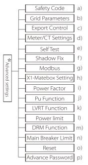
All advanced settings can be set here, such as battery, grid, off-grid, etc.. "Advanced" setting is generally customization and resetting for battery and grid . Each part has lower level parts. Please contact your installer or factory and enter the installer password.
