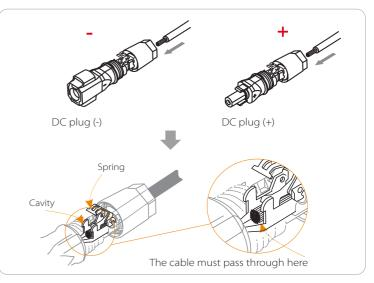
Step 3. Press down on the spring by hand, you can hear a click sound , then push the ends together, and tighten the screw joints.
