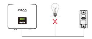
Figure: Wrong connection of load and inverter
