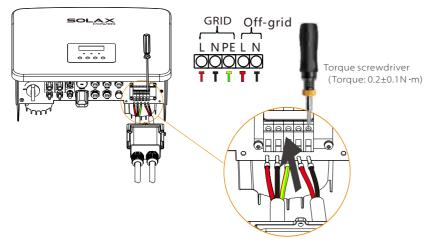
Step 5. Install the AC waterproof cover, and tighten the screws on the four sides of the waterproof cover with an Allen wrench.
