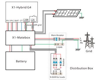
Diagram C: Neutral line and PE line are combined togeter, and the common load is connected to the off-grid port; (Apply to Australia)
