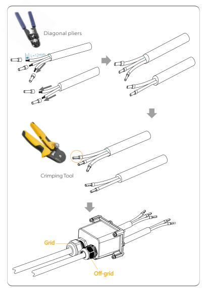
Step 4. Find the location of the AC interface on the inverter, insert the crimped terminals into the UW10 terminals L, N, and P according to the wire sequence, and use a flat-blade screwdriver to tighten the screws. (Torque:  $0.2\pm0.1N \cdot m$ )
