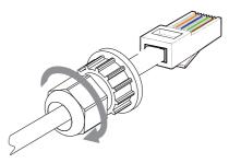
Step 5: Finally, find the corresponding COM, METER, CT, DRM ,LCD poets on the inverter and insert the communication cable into the corresponding ports.
