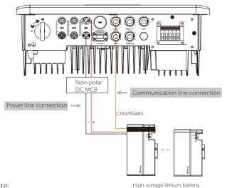
Note: High voltage lithium battery When using SolaX batteries, it is recommended that the number of battery control (T-BAT-5.8) is 1 and the number of battery modules (HV11550) is 1-3; the number of battery control (MC0600) is 1 and the number of battery control (HV10230) is 1-4 pcs.
