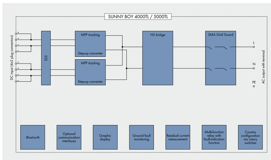
Block circuit diagram of a multi-string inverter without transformer
