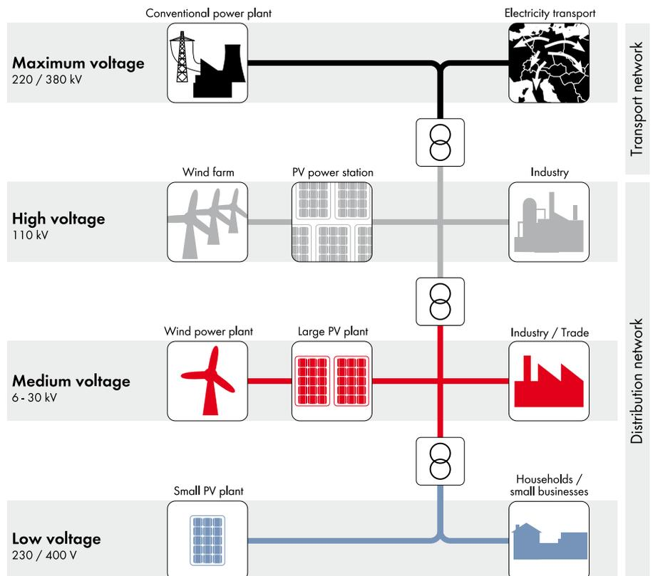
The grid levels in the AC power distribution grid
