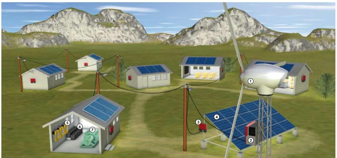
**Components:** 1. Wind turbine system, 2. WINDY BOY, 3. SUNNY BOY, 4. Solar generator, 5. SUNNY ISLAND, 6. Batteries, 7. Diesel generator
